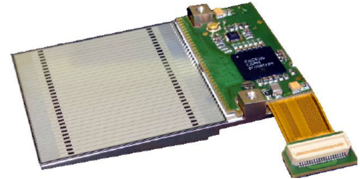
1 sensor contains 32 silicon strips
