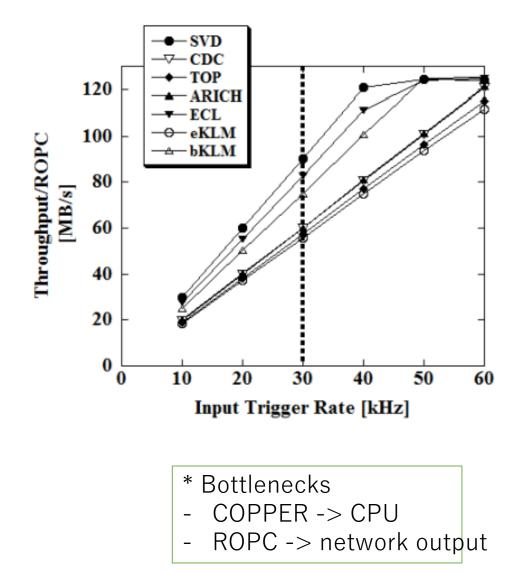
Throughput is saturated due to the limit of output GbE bandwidth.
