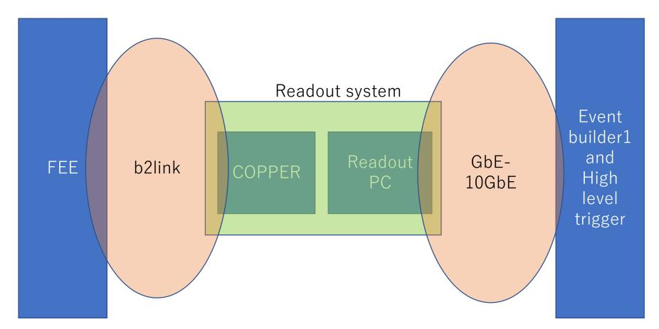
Basic framework of belle2link (Rocket-IO based serial link) should be the same. Otherwise FEE's FW/HW update might be needed.
